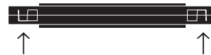
The latch on the left corresponds to recordings on side 1 (A), and the latch on the right corresponds to recordings on side 2 (B).
