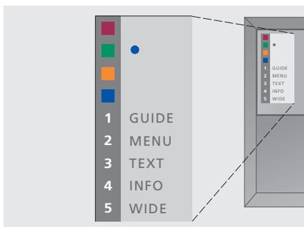
*Example of a Set-top Box Controller menu – The Beo4 buttons are shown to the left on the menu and the set-top box buttons are shown to the right.*
