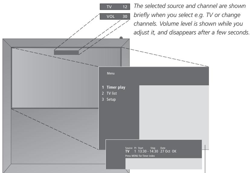
The selected source and channel are shown briefly when you select e.g. TV or change channels. Volume level is shown while you adjust it, and disappears after a few seconds.
