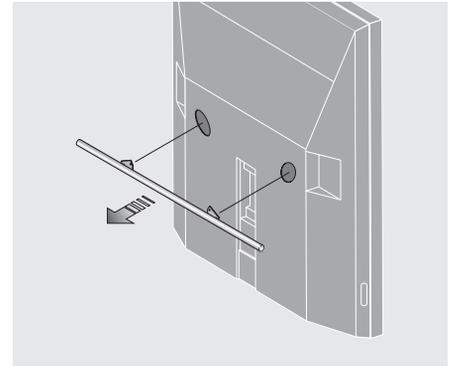
*Before placing BeoVision 5 you must remove the handle.*
