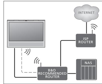
Example of recommended network setup either wired or wireless.
