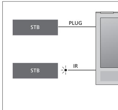
**IR-transmitters:** To operate non-Bang & Olufsen products with a Beo4/Beo6 remote control, attach a Bang & Olufsen IR-transmitter on your non-Bang & Olufsen product and then connect it to one of the sockets marked PUC on the connection panel. Attach the transmitter near the IR-receiver on the connected equipment to ensure remote control operation. Before attaching it, check that you can operate the equipment menus on the television screen using the Beo4/Beo6 remote control.
